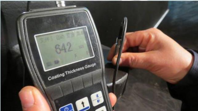
One layer anti-rust priming coating and more than two layers finishing coating. This photo shows coating thickness inspection.
