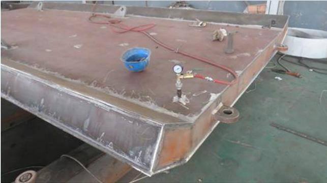
Checking each weld joint carefully make sure there is no solder skips, incomplete weld and other phenomena.
