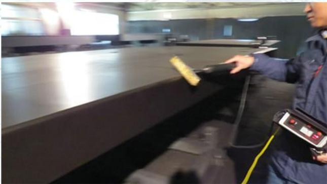
Detecting the dew point of the spray-paint, and checking the strength of the paint coating.
