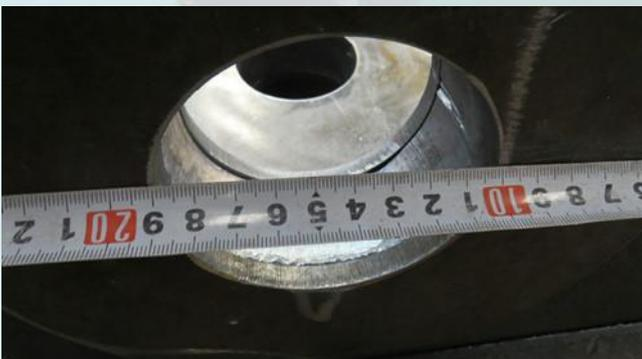
Measuring each part to ensure that the products meet the requirements of design drawings. At the same time, correcting the wrong welding parts.
