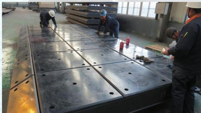
Mounting PE face pads on the steel frame.
