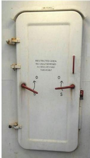
As the name implies **weathertight door** is a kind of marine door which is required to be installed at the entrance of both ends of the enclosed superstructure above the freeboard deck. Most of them are made of steel and aluminum alloy material. Its structure is similar to that of a hinge-type watertight door, but the door leaf is thinner and the number of door clips is less. It can ensure weathertight only.
